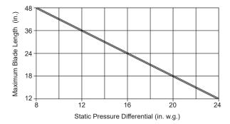
This damper's design at a blade length of 48" has a maximum allowable blade deflection of L / 360 for the static pressure indicated on the chart. At reduced blade lengths, higher static pressure limits can be attained without sacrificing damper operating performance characteristics.
